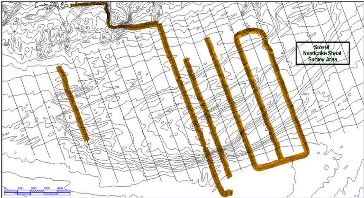
Figure 4-5. Reconnaissance sidescan sonar lines acquired over the Maitland Ridge fall 2011. For comparison, the rectangle in the upper right portion of the figure represents the size of the Nanticoke Shoal survey area.
