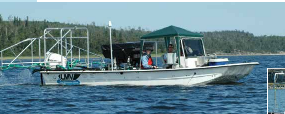
An innovative granular bayluscide sprayer boat employs a high pressure spray system and GPS to effectively target lentic areas on the St. Marys River system.
