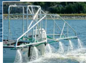
An innovative granular bayluscide sprayer boat employs a high pressure spray system and GPS to effectively target lentic areas on the St. Marys River system.
