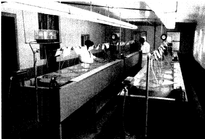
Constant temperature baths utilized in conducting bioassay tests. The four independently controlled baths shown can hold 68 ten-liter test jars.
